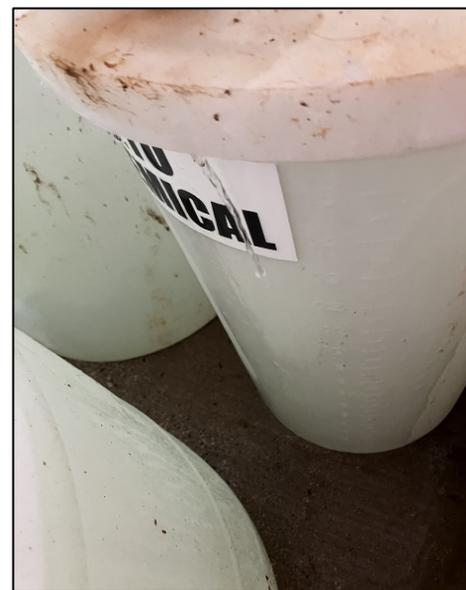
*Pictured above at left is a container of FutureCow test strips. Above at right is a picture of water dripping from a FutureCow mixing barrel from a stuck float adding too much water.*
